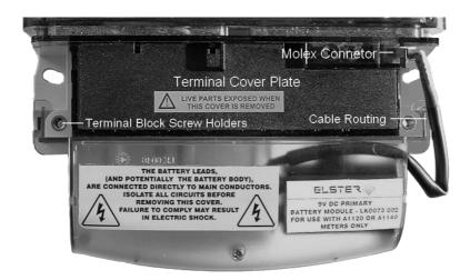
An External Battery Module can be fitted as an option which allows reading of meter data via the optical port and access to the display facilities during power outages. The battery is housed in the Module Carrier that fits below the meter terminal cover.
